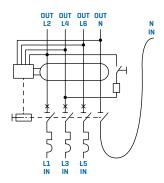
Will operate and is suitable for 4 wire motor circuits without the load neutral
